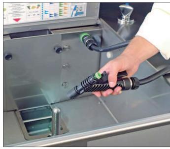
The inside is designed for easy cleaning: with rounded corners and completely accessible. We've thought of everything: there is even a water outlet so you can plug in a water jet for thorough cleaning.
