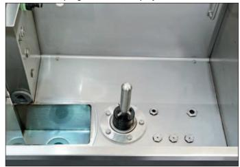
This is what hygiene really looks like: stainless steel inside, rounded corners and edges, water jets at the bottom and at the sides, also made from stainless steel. Everything is easily accessible, no need for special tools if you want to take it apart for thorough cleaning.
