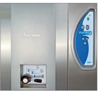
Using the machine is simple: choose your program with the plus/minus button, then choose the washing intensity that's it! One more thing .... don't forget to remove the produce after 7-12 minutes!!!
