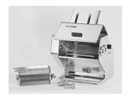
The MST Meat Tenderiser is finished throughout in stainless steel. Electric motor drive. The appliance requires no servicing or maintenance. The cover is available in a selection of stainless steel or in transparent plastic.
